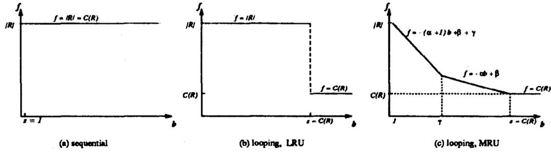
Figure 2: Faulting Functions of Sequential and Looping References
