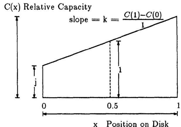
Figure 1: Model of Distribution of Storage Capacity
