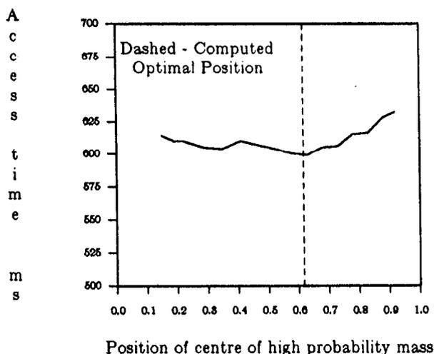
Figure 9: Measured cost for position of P1 group
