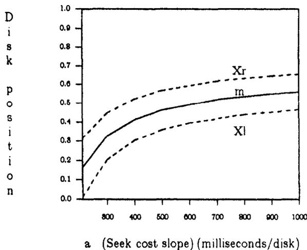
Figure 5: Optimal Position as function of seek slope
